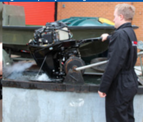
Engine running and underway (within 10 seconds of being righted)
