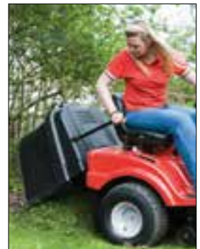
Left: 46 cm / 18" turning radius for very good manoeuvrability working around trees or in confined spaces. Above: Mowing deck with antiscalp wheels to prevent damage to the grass surface. Right: All tractors with rear discharge have a grass catcher which is easy to empty from the driver's seat.
