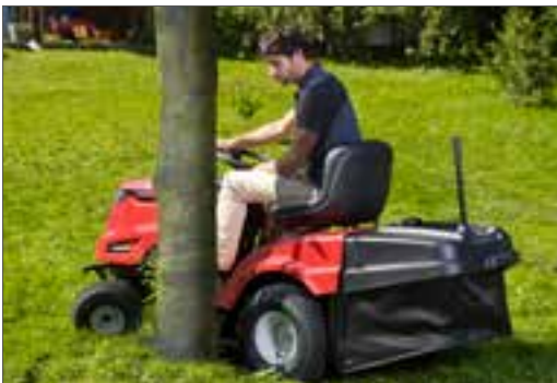
Left: 46 cm / 18" turning radius for very good manoeuvrability working around trees or in confined spaces. Above: Mowing deck with antiscalp wheels to prevent damage to the grass surface. Right: All tractors with rear discharge have a grass catcher which is easy to empty from the driver's seat.
