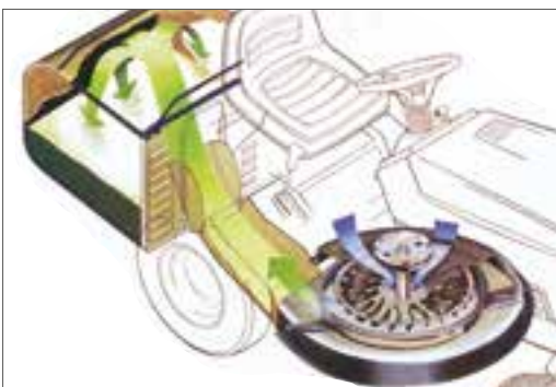
Left: "Direct Collect®" A large turbo fan assister, coupled with the heavy duty cutter blade, physically throws and blows grass cuttings, leaves and other debris directly into the large capacity collector. (on model 603RT) Above: Anti scalp wheels Right: Shift-on-the-go with continuous variable shifting
