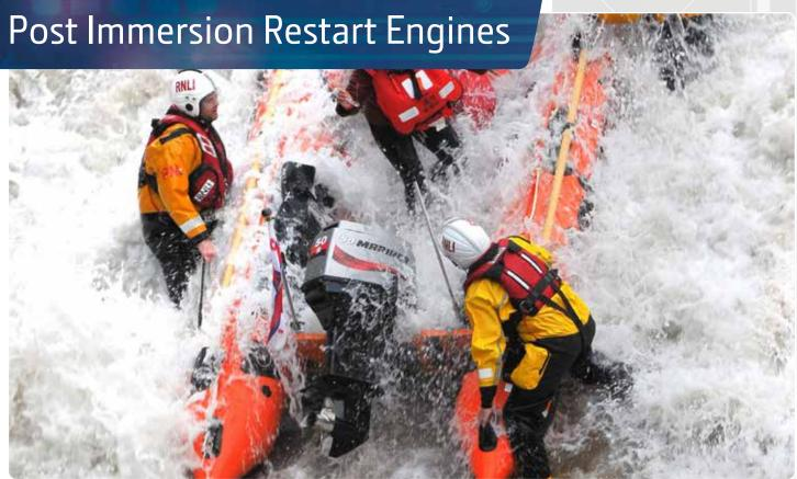
PIRS (Post Immersion Restart System) restarts an outboard engine after being submerged; a system designed and developed by Barrus for the military, commercial and rescue services.
