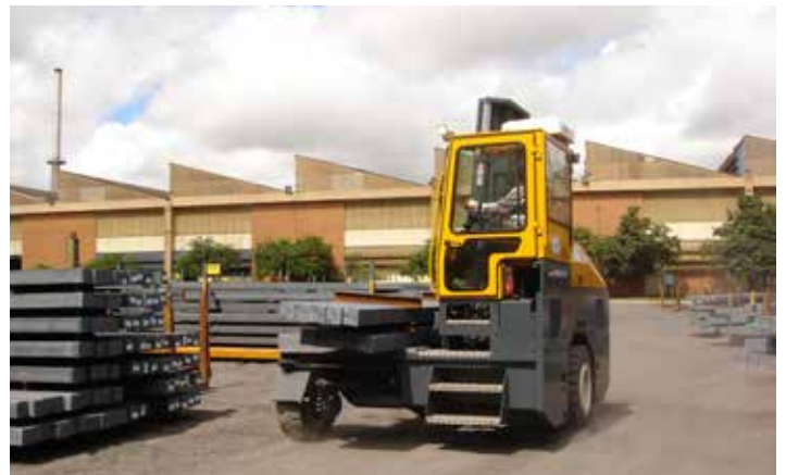
The high ground clearance of the C14,000 is ideally suited for both indoor and outdoor use.
