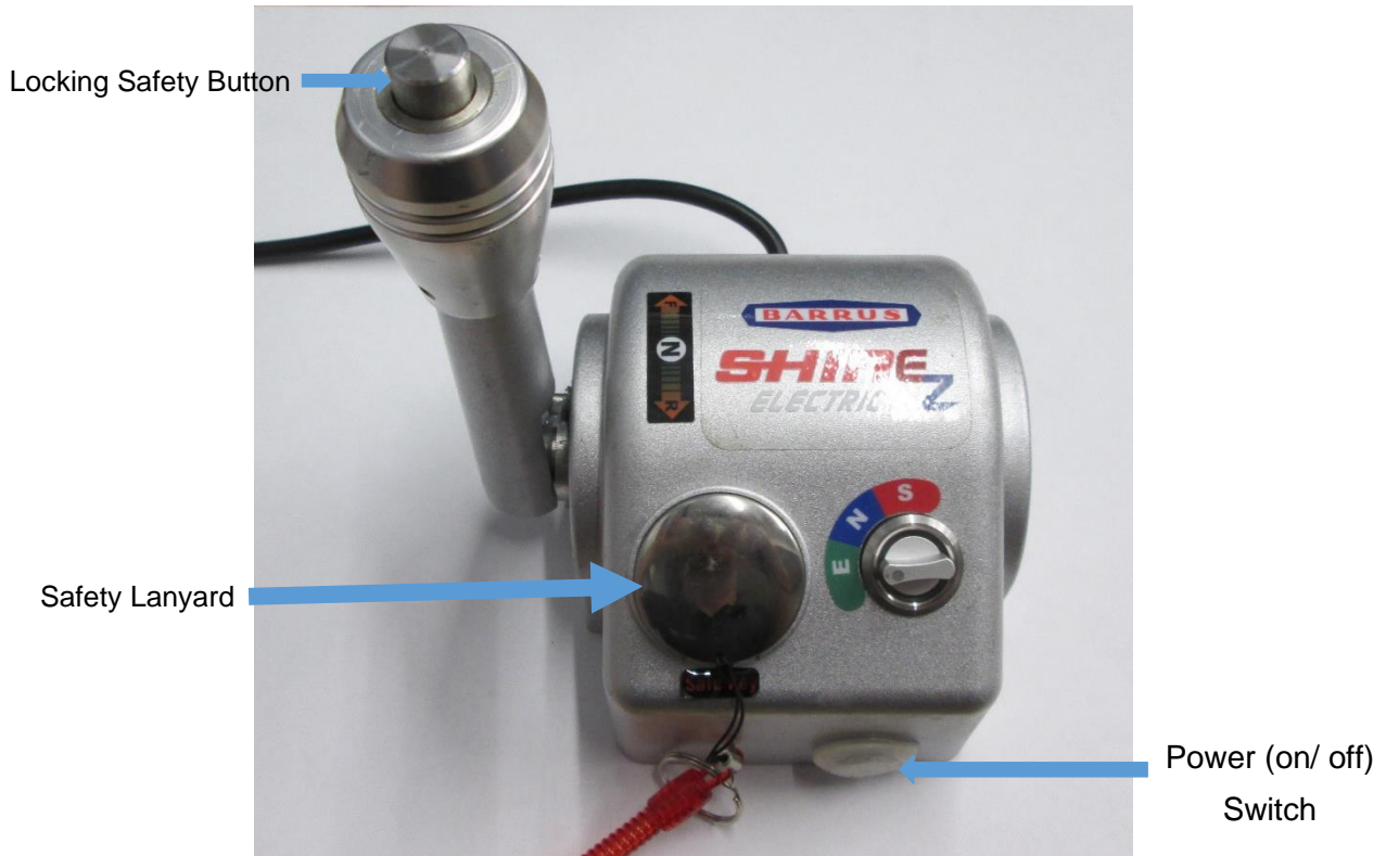
Figure 13: Safety Lanyard attached to control lever
