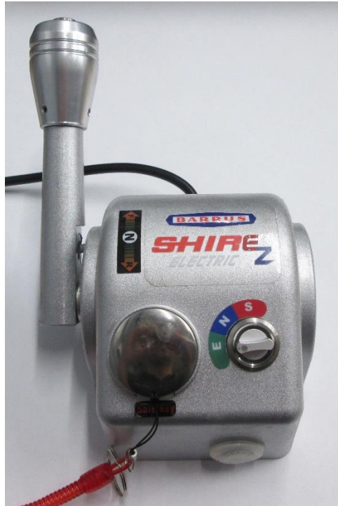
Figure 14: Speed and Direction Control Lever in forward position
