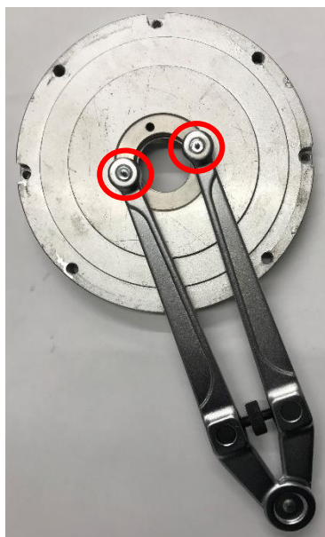
Figure 24: How to use Motor Front Bearing/Seal Removal Tool
