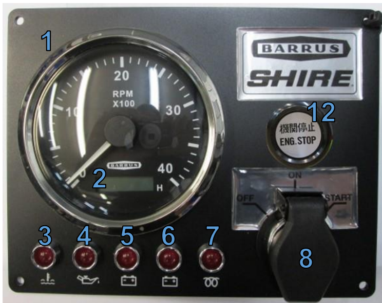
Figure 15: Standard Control Panel
