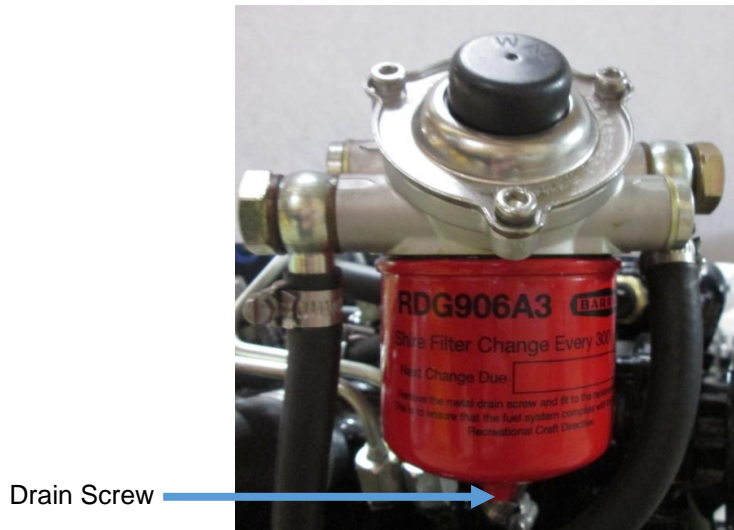
Figure 33: Fuel Filter Drain Screw
