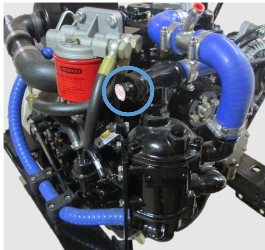
Figure 34: Work Boat Anode Location
