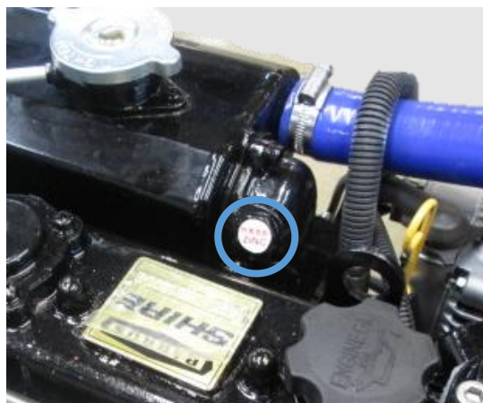
Figure 35: River Boat Anode Location
