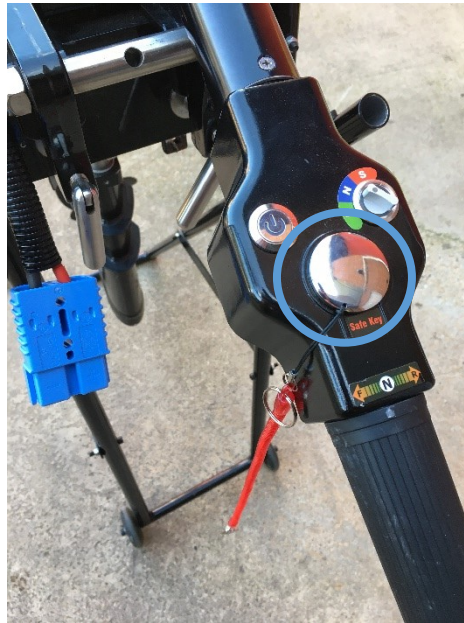
Figure 29: Safety Lanyard attached to the stop switch
