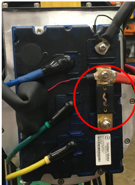
Figure 27: Fuse Position on a S10 Engine
