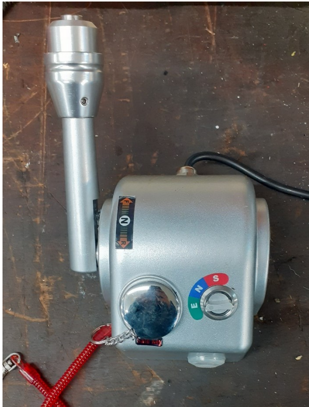
Figure 31: Speed and Direction Control Lever in forward position
