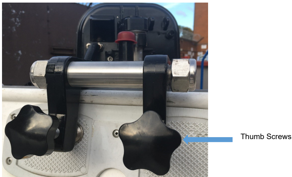
Figure 16: Fitting outboard to boat
