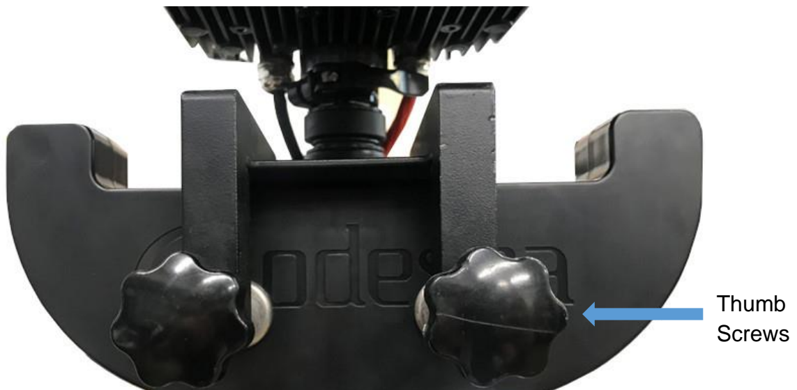
Figure 13: Fitting outboard to boat
