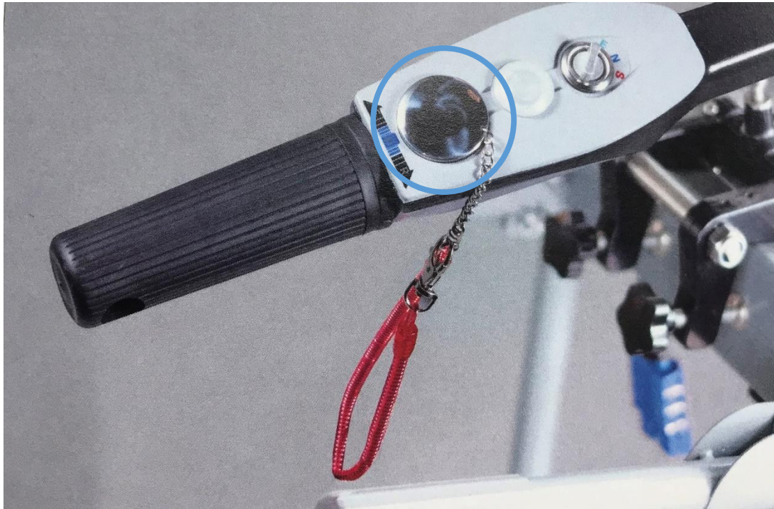
Figure 27: Safety Lanyard attached to the stop switch
