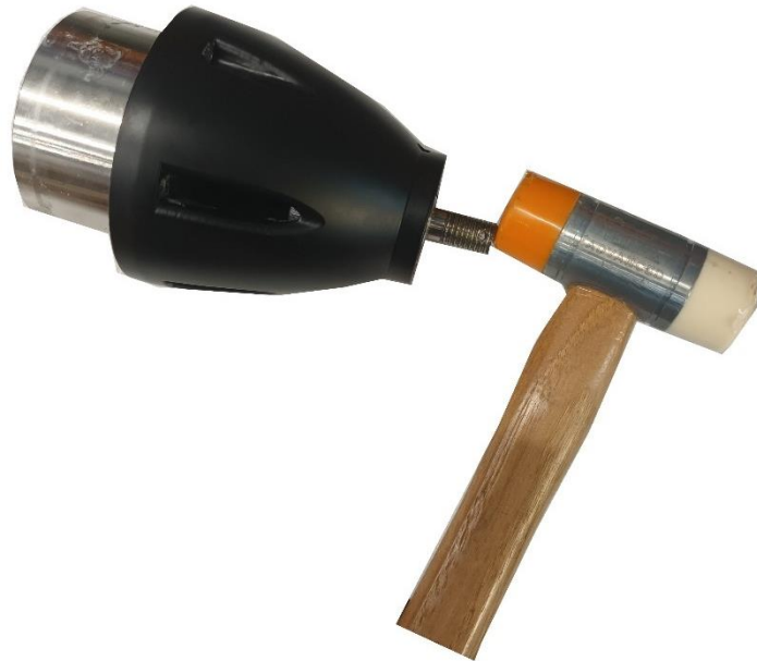
Figure 47: Disassembling Prop Shaft Assembly
