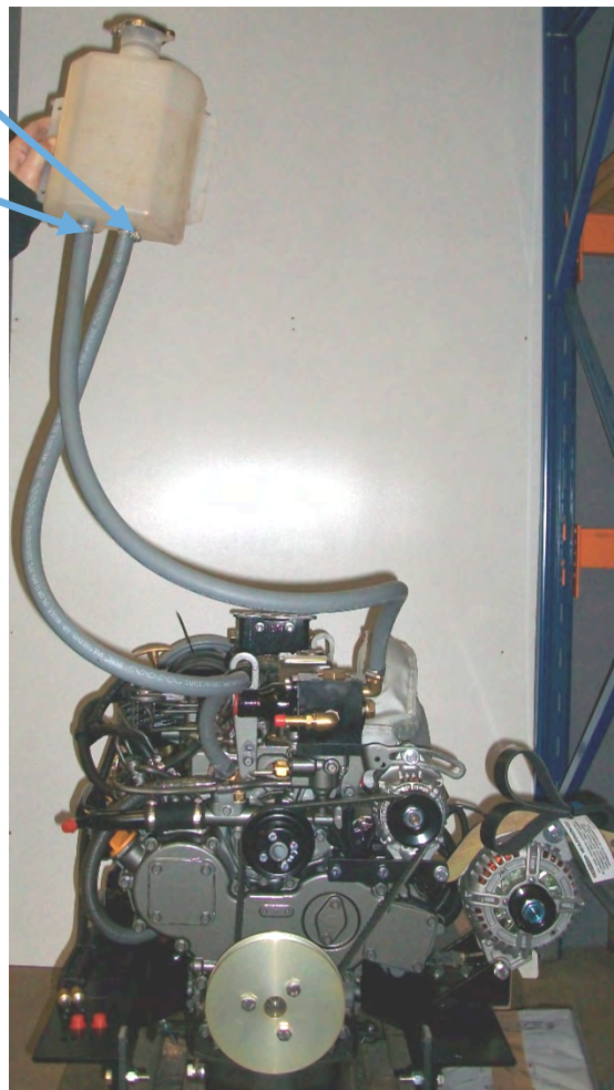
Figure 5: Shire 40 Header Tank Connections
