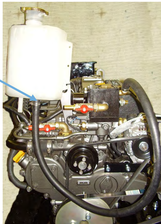
Figure 7: Shire 50 Header Tank Connections
