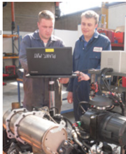
Pictured left to right: Paul Hambleton and Tom Burton, Level 2 Construction Plant Maintenance Apprentices using Smartassist to diagnose system faults on Yanmar Tier 4 engine.
