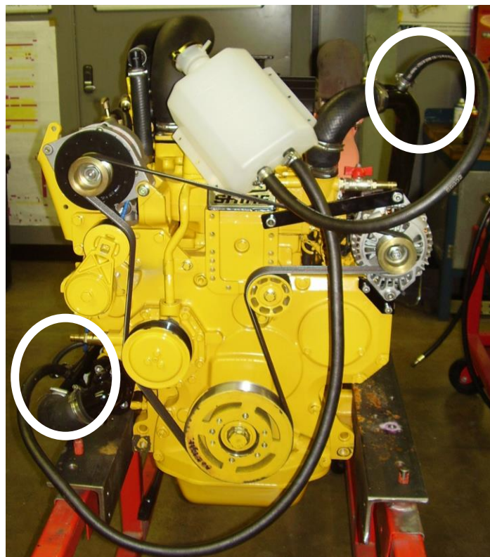
Figure 3-3: Shire 90 Header Tank Connections
