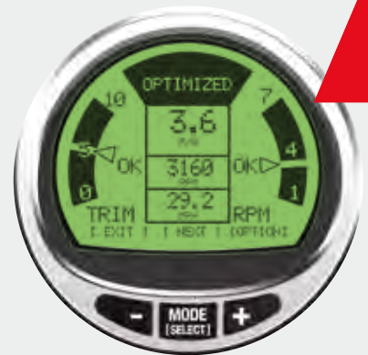
MercMonitor displaying ECO-Screen
