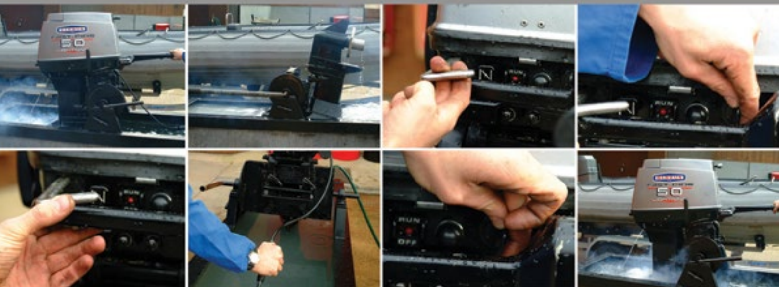
Electric restart procedure shown.
