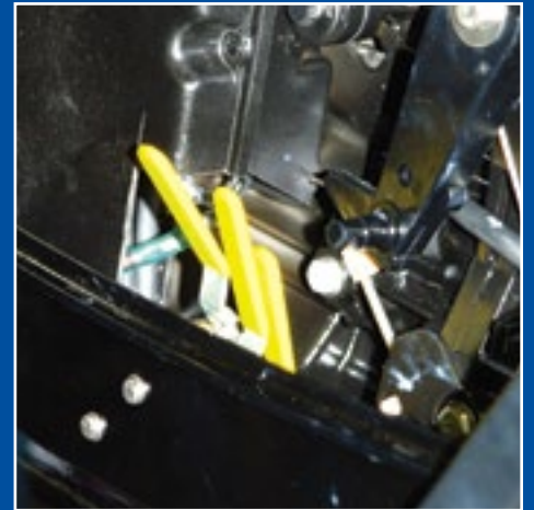
PIRS drain taps shown on 50hp engine.
