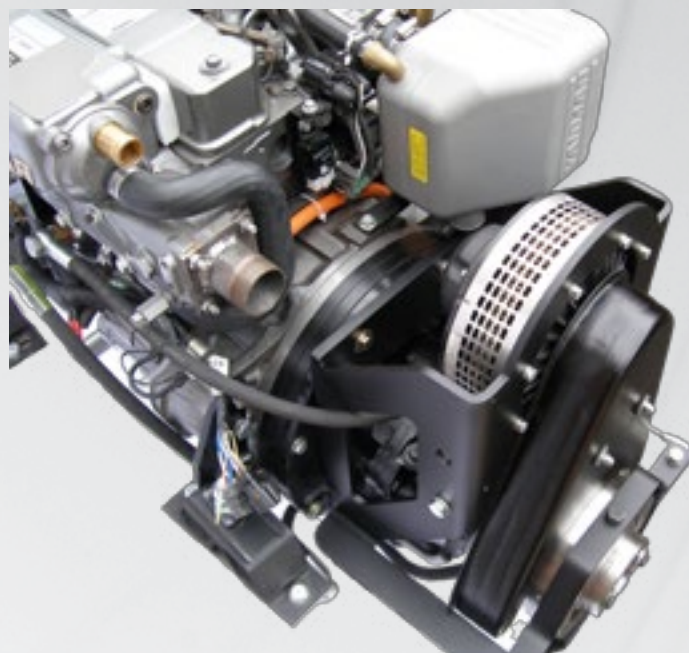
Yanmar 4JH5E (54hp) Hybrid with 10kW electric motor
