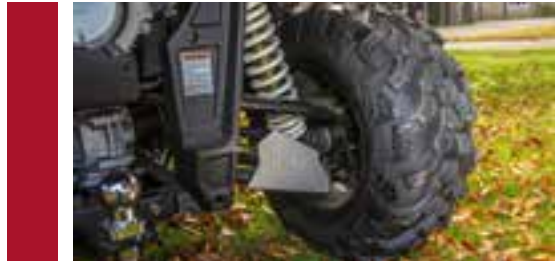
Independent dual A-arm suspension front and rear
