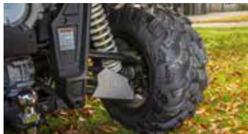
Independent dual A-arm suspension front and rear
