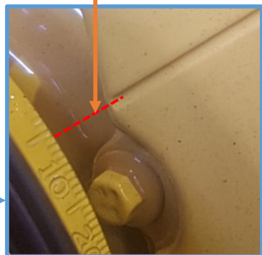
Timing marks lining up at 6° btdc with cylinder number 1 in compression
