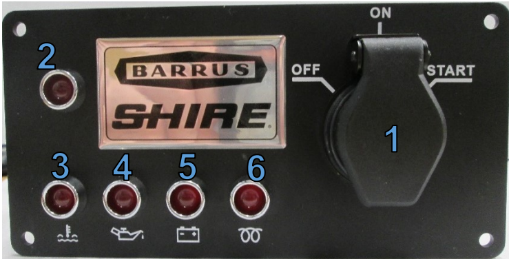
Figure 8: Basic Control Panel (Twin Alternator Engines)
