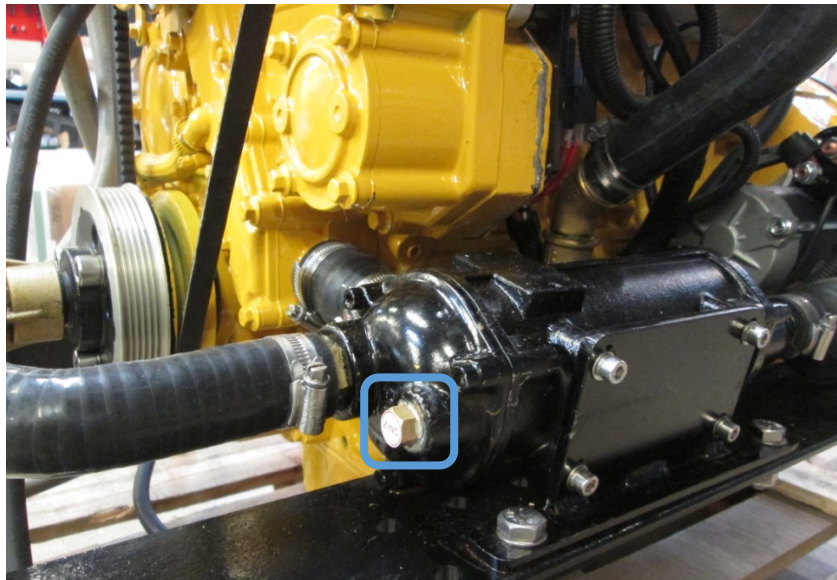
Figure 20: Work Boat Anode Location
