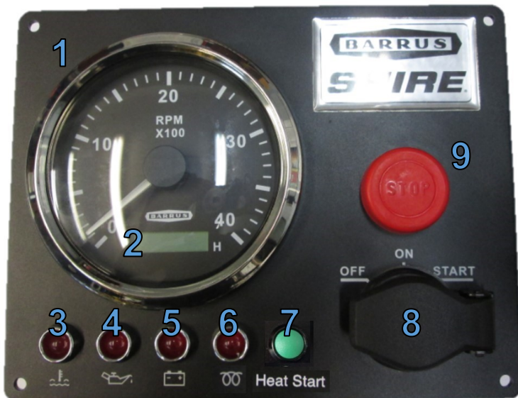
Figure 14: Standard Control Panel
