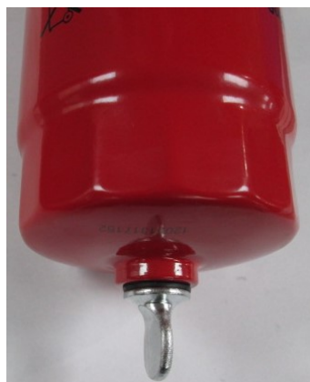
Figure 17: Primary Fuel Filter Drain Screw
